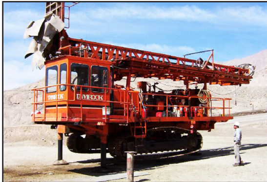
Drifters drill holes to set explosive charges for excavation of copper ore.
